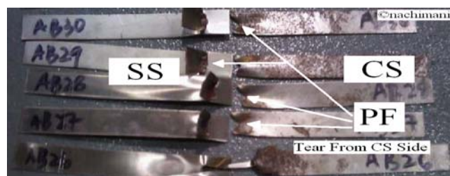
Figure 5(c). Tear from one side (PF) failures in group
