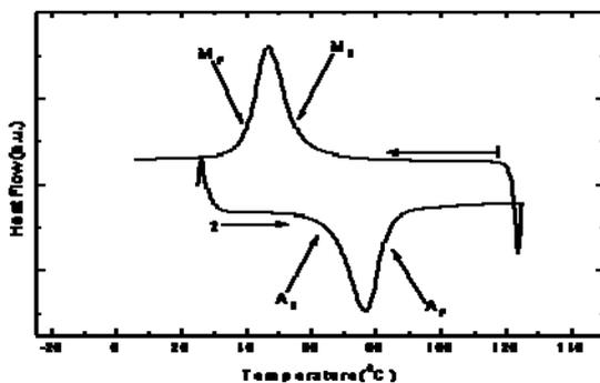
Figure 5. Martensitic transformation for sample  $Ni_{50}Mn_{37.5}Sn_{12.5}$
