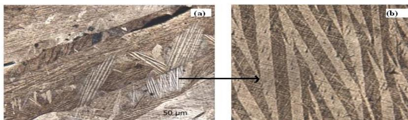
Figure 2. (a) A number of Martensitic layers present in  $Ni_{50}Mn_{45}Sn_5$ , (b) enlarged martensitic layer at 20X magnification
