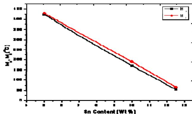
Figure 6. Comparison of  $M_s$ ,  $M_f$  with respect to Sn weight percent
