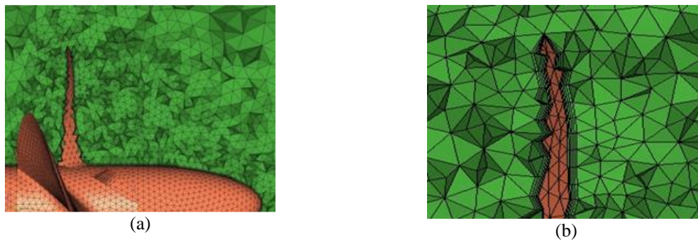
Figure 2. Type of mesh surrounding propeller blade of (a) Prism elements and (b) Mesh connectivity
