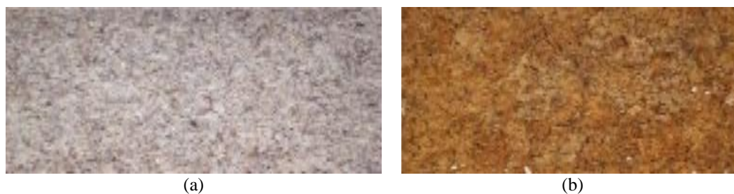
Figure 2. Grinded rubber seeds by (a) before been placed in oven and (b) after been placed in oven
