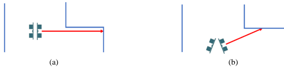
Figure 11. Distance measurement via ultrasonic sensor (a) horizontal and (b) oblique distance measurement
