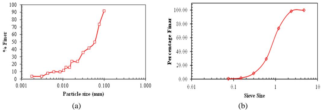
Figure 3. Particle size distribution curve of (a) SCA and (b) BF-slag
