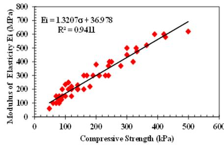
Figure 11. Correlation between initial tangent modulus and compressive strength
