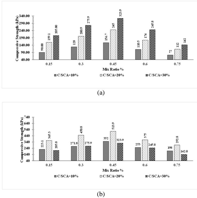
Figure 7. Compressive strength of materials for (a) 7 days and (b) 28 days
