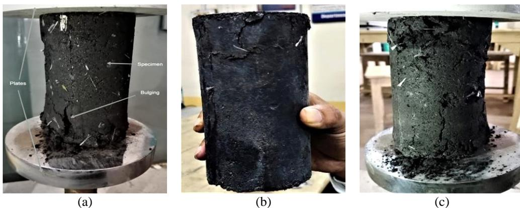
Figure 5. Cylindrical specimen inflation and crack development of (a) specimen inflation, (b) cracks in the specimen, and (c) cracks and specimen inflation
