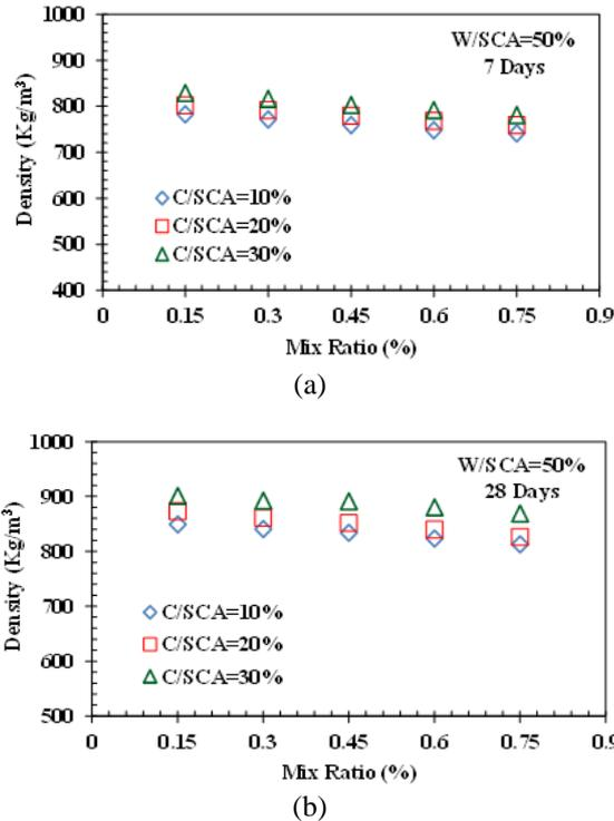
Figure 6. Density of materials for (a) 7 days and (b) 28 days
