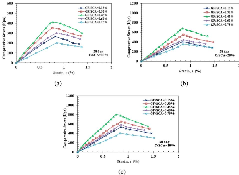
Figure 10. Stress-strain curve of SCA and BF-slag under compressive stress for 28 days of (a) C/SCA=10%, (b) C/SCA=20%, and (c) C/SCA=30%
