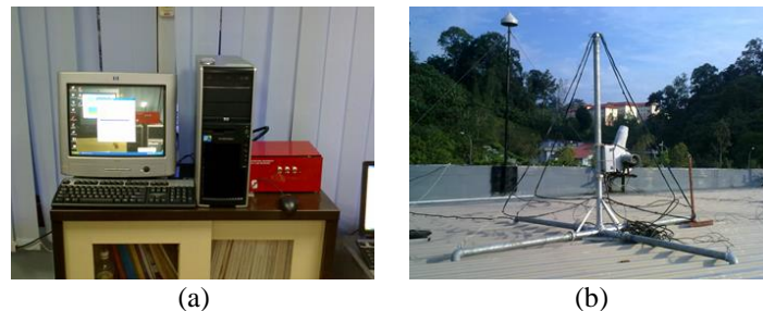
Figure 3. System setup consists of (a) a receiver (indoor) and (b) a VLF antenna (outdoor)
