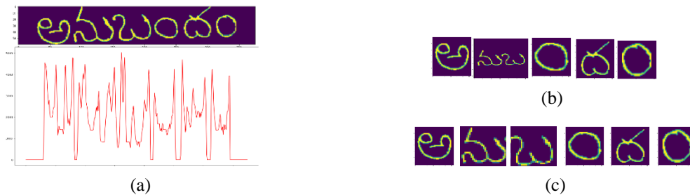
Figure 1. Segmentation of word in (a) histogram of the given word, (b) separation of characters based on spacing, and (c) segmented characters after applying segmentation algorithm
