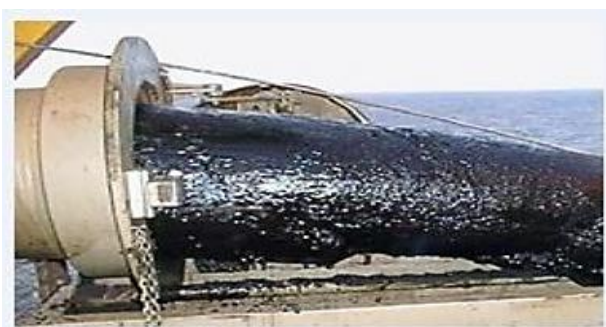
Figure 1. Wax blockage in subsea pipeline [9]
