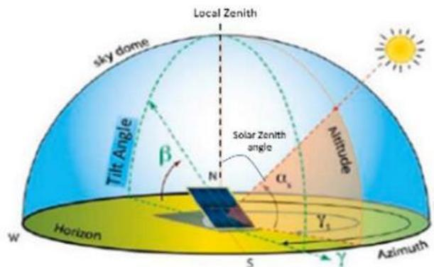
Figure 2. Reality of solar tilt, azimuth angle, and solar zenith angle orientation
