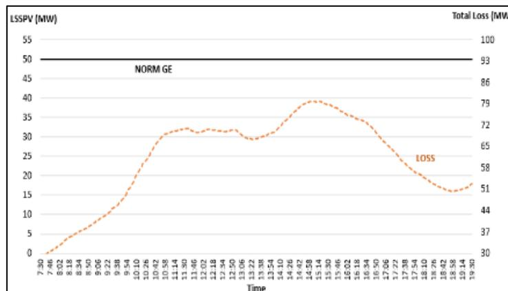
Figure 8. Nominal constant generator 50 MW integrated at bus two and the result of losses
