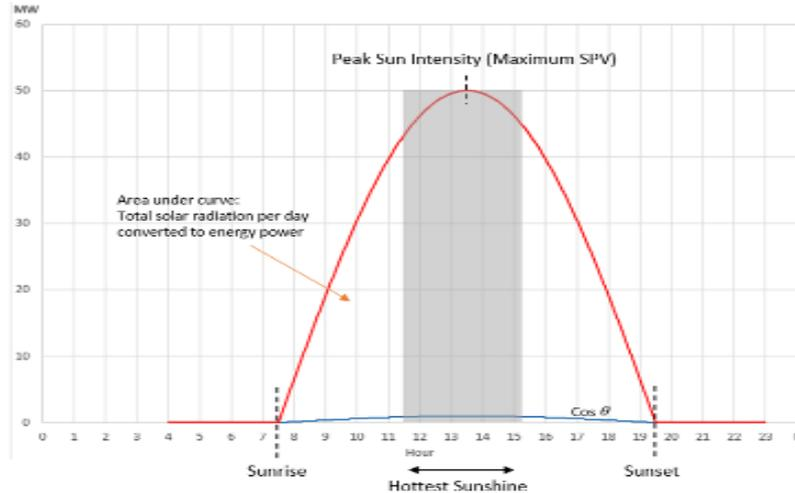
Figure 3. New typical daily SPV generation (TYP) forecasted suitable used in simulation network
