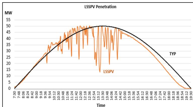
Figure 4. Profiles for typical (TYP) and LSSPV generation
