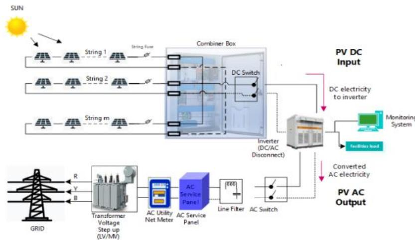
Figure 1. The schematic diagram for LSSPV in Malaysia
