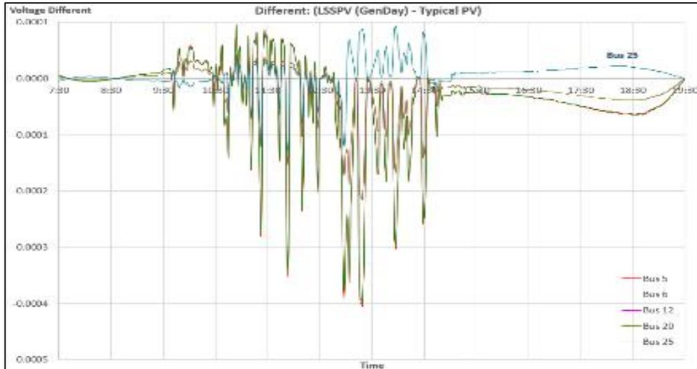
Figure 4. Difference voltage fluctuation occurs between LSSPV and typical SPV
