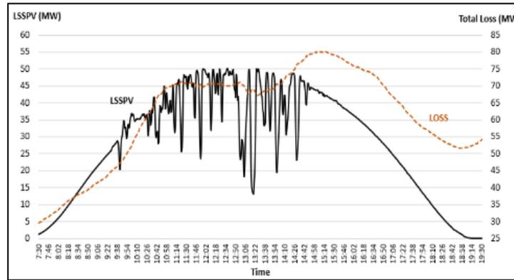
Figure 3. LSSPV and its losses in profile pattern
