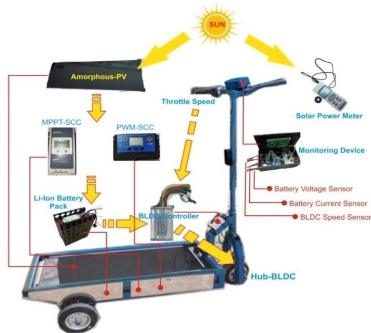
Figure 1. Experimental setup for comparing solar charger controller (SCC) types on E-scooter battery charging
