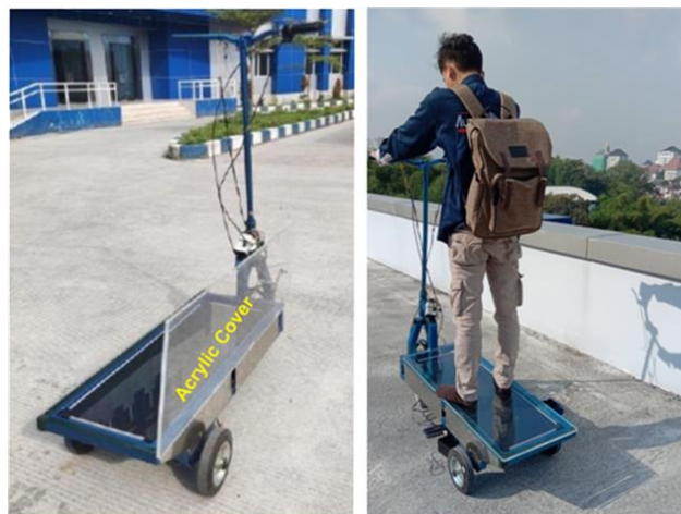
Figure 3. The prototype solar-powered three-wheel electric scooter [33]
