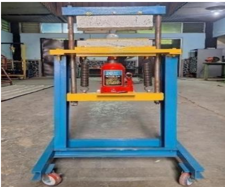
Figure 3. Hydraulic jack system bending tool
