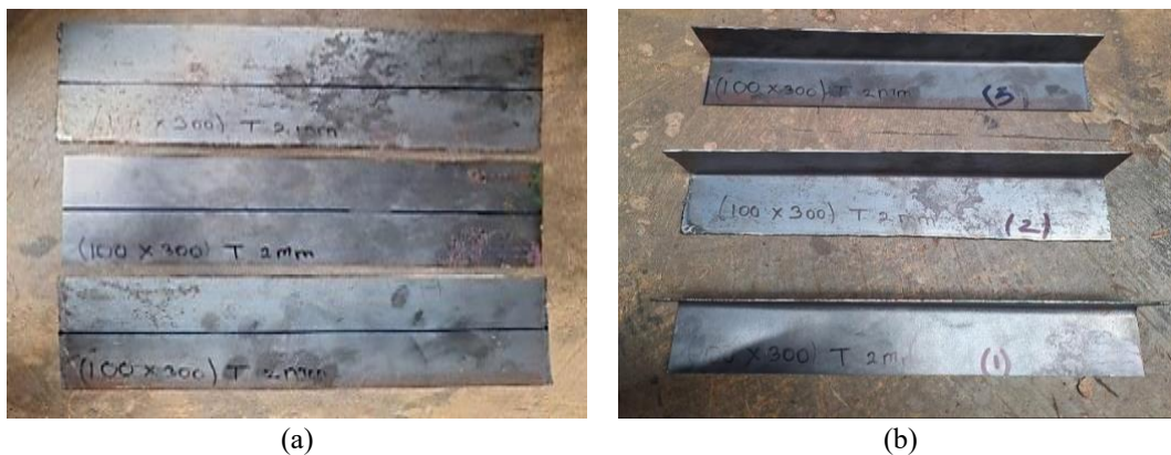
Figure 6. Comparison of bending samples of (a) sample before bending and (b) sample after bending
