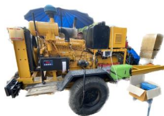
Figure 2. A Hino EH100 diesel engine with a capacity of 5,871-cc coupled to a 60-kW alternator
