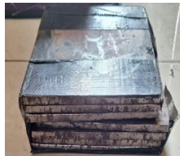
Figure 1. AH36 steel specimens for mechanical testing
