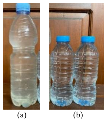
Figure 3. Comparison of bore well water samples of (a) before and (b) after filtration
