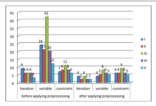
Figure 1. Comparison of Number of Iterations, Variables and Cosntraints Before and After Applying Preprocessing and Probing Techniques
